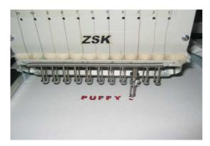
2. Put PUFFY in place, fix with little adhesive spray if necessary (e.g. caps)
