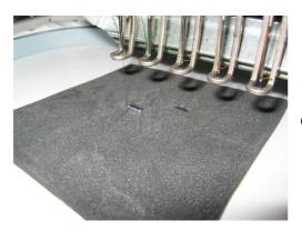
column stitches rotated by 90° to support the perforation.
